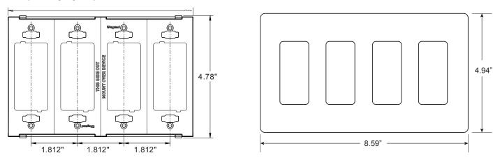
Align subplate over NEMA 26 sized electrical devices and receptacles. Affix subplate with included screws to electrical wall box. Secure tightly, but avoid over torquing screws. Snap on radiant screwless wall plate to subplate.
